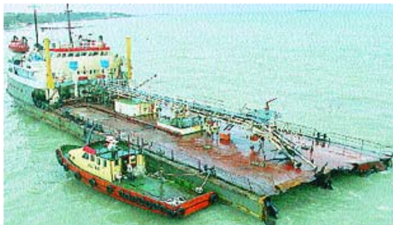
Figure 10. Russian Tanker Volganef-248 Split into Two Pieces on the Coast of Florya
